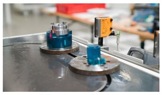
Each working stage in the automatic lathe requires a custom jig. The jigs are attached to the conveyor belt using standard shuttles.
