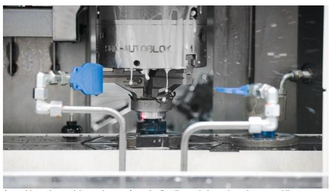
A machine gripper picks up the part from the first jig, and places it on the second jig once the machining process is complete.
